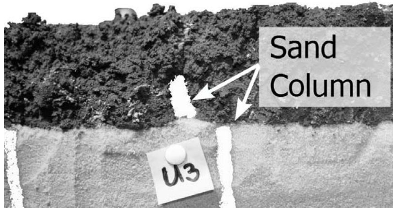
Figure 5. Photograph of strain concentration in the sand immediately below the clay crust on the non-treated side of the model shown in Figure 3 (Boulanger et al. 2012).
