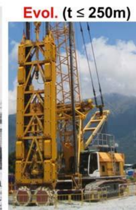
Figure 20. Advances in Geotechnical Engineering 1936 - 2011: "From Revolution to Evolution". Slurry trench wall as an example of technology.
