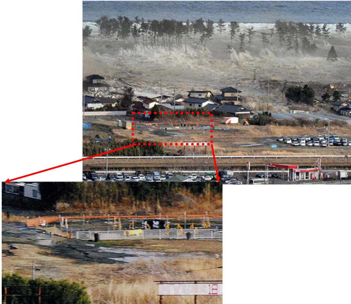
Evidence of liquefaction before the tsunami struck. (Motoki Kazama, Tohoku University from Japanese Geotechnical Society (JGS) website : first results of its activities after the occurrence of the 11th March, 2011 Tohoku earthquake, http://www.jiban.or.jp/e/disaster-survey-information-of-2011-tohoku-earthquake-2/ )
