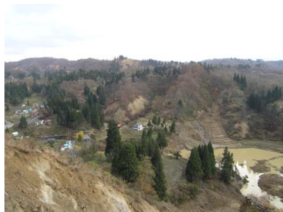
Fig. 20 Houses located on safer parts of seismically affected slope (Yamakoshi Village, after 2004 Niigata-Chuetsu earthquake, Japan).
