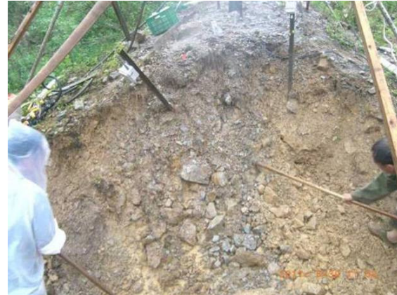
Fig. 20 Rainfall-induced failure of a cut slope.
