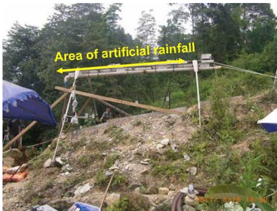
Fig. 19 Artificial rainfall on slope in Sichuan Province, China.
