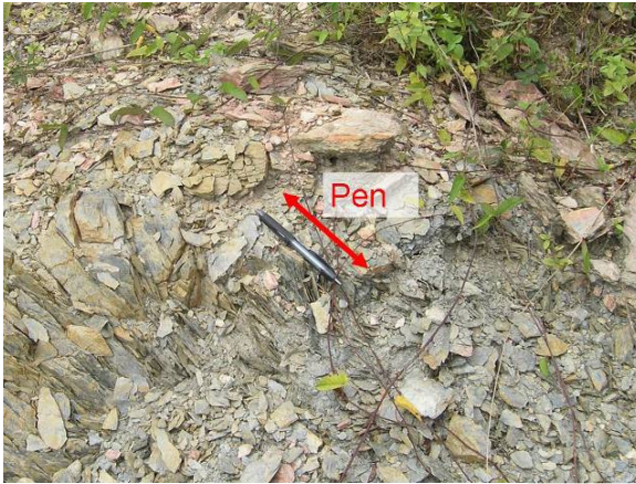
Fig. 11 Breakage of Phyllite rock by weathering and water action.
