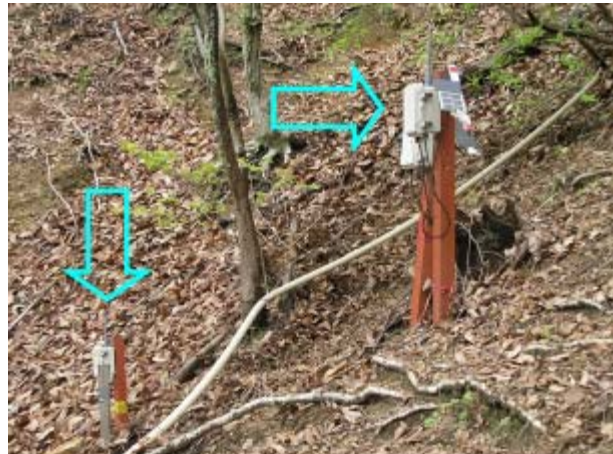
Figure 3. Inexpensive early warning device for slope failure during heavy rainfall
