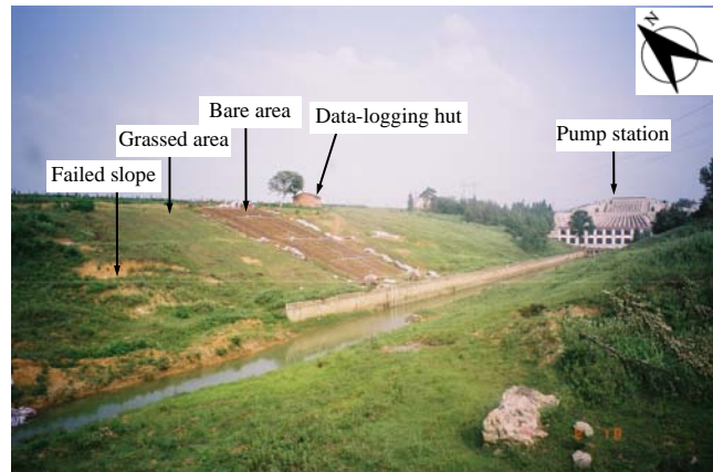
Figure 5 General layout of the test site in Zaoyang for preliminary field study
