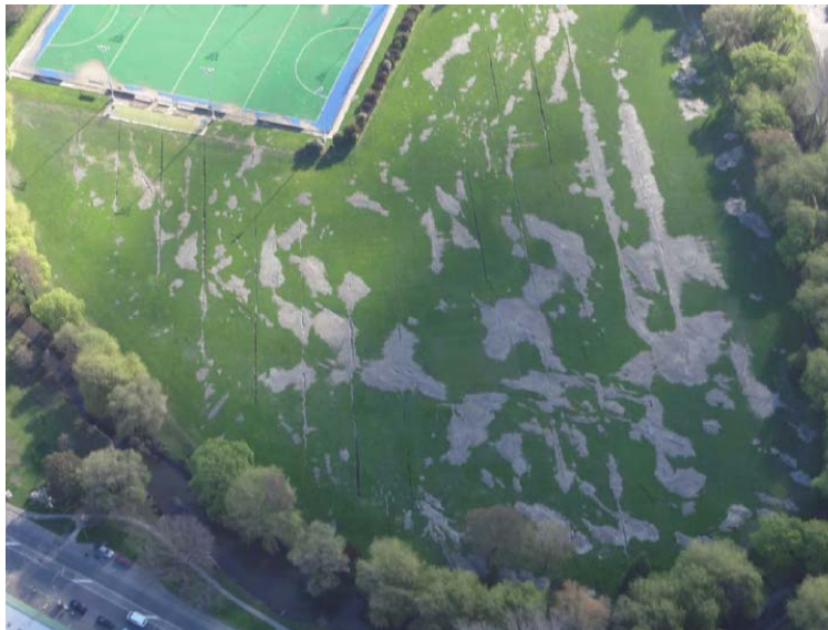
Figure 5. Evidence of extensive liquefaction (large sand boils) in Porritt Park, Christchurch. Using the vehicles (bottom of photo) or the hockey field (top of photo) for scale gives a good indication of the significant volume of sand ejecta.
