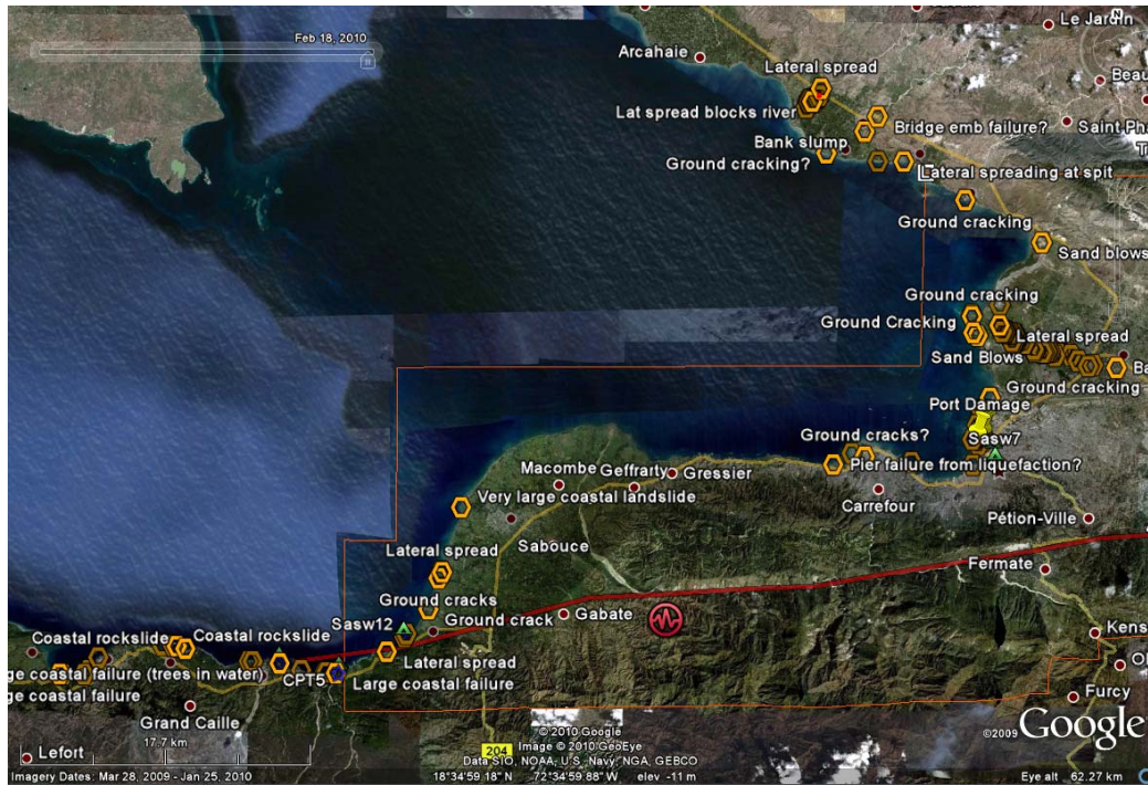
Figure 10 Liquefaction, lateral spreading, and coastal failure sites identified from post-earthquake aerial photography (sites identified as open hexagons)
