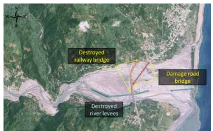
Figure 31. Damages in bridges and river levees
