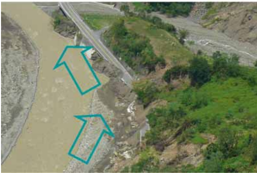
Figure 17. Toe erosion in river channel
