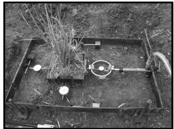
Fig. 4 Field direct shear test equipment
