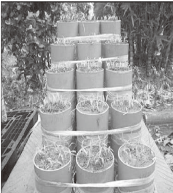
Fig. 1 Planted grasses in PVC mold for laboratory tensile test
