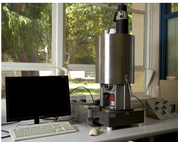
Figure 6. New generation of UWA simple shear apparatus
