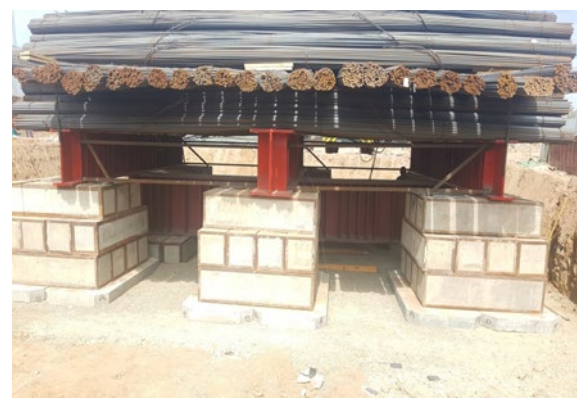
Fig. 2. Static load test in construction site LRT-Astana.
