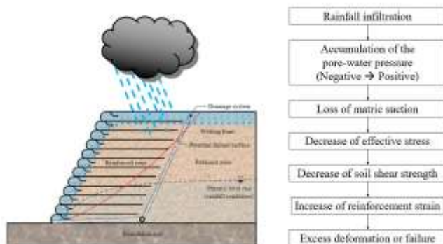
Figure 1. Failure mechanism of GRS structures under rainfall conditions
