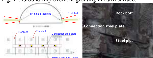
Fig. 13. Reinforced steel pipes in sidewall.
