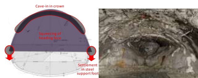
Fig. 6. Difficulties encountered in the silt layer section.
