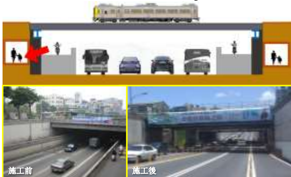
Figure 8. Cross-section of the Zhonghua 3rd Road underpass
