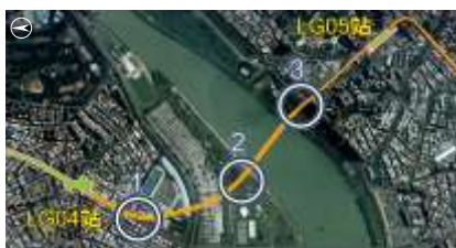
Fig. 2. The route design in original plan (three curves)
