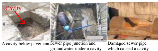
Fig. 2. Photos at detail investigations of cavity and a broken sewer pipe by aging which caused a cave-in.
