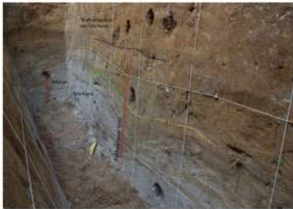
Fig. 7. Indication of Pauh fault on the palaeoseismic trench wall.
