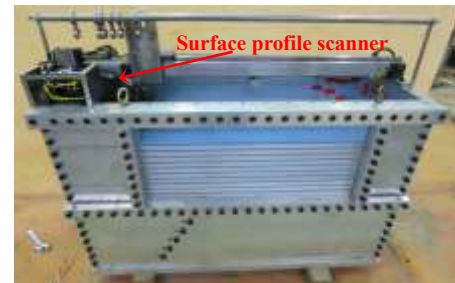
Fig. 4. Fault simulation container equipped with a surface profile scanner and sand bed with dyed sand layers before test
