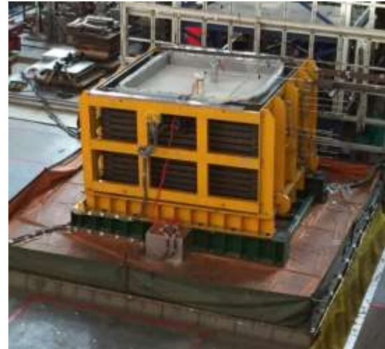
Fig. 2. Finished model of the shaking table test.
