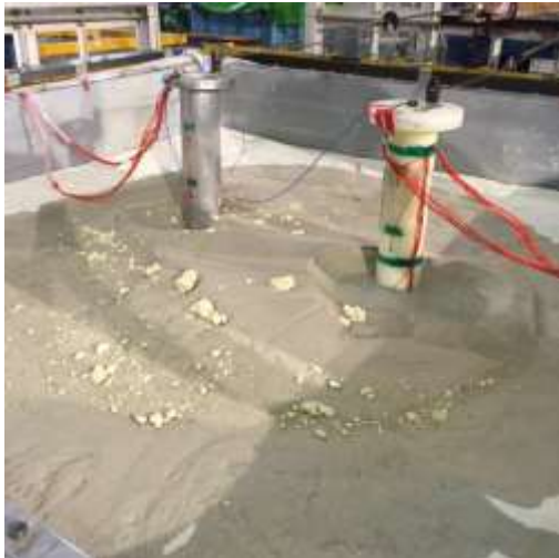
Fig. 4. Soil surface condition after shaking.
