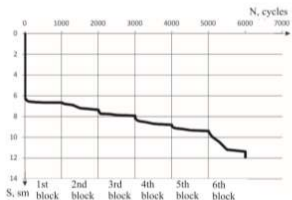
Fig. 12. Base deformations under regime cyclic loading.
