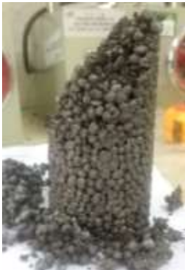
Fig. 5. Cemented LECA specimen after failure in monotonic unconfined compression test
