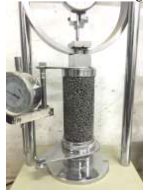
Fig. 3. Unconfined compression test on cemented LECA
