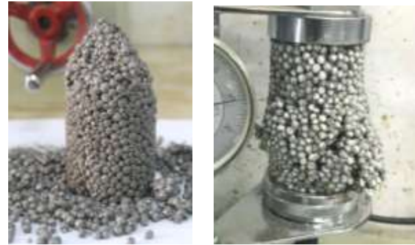
Fig. 9. Failed specimens in monotonic loading.
