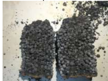
Fig. 7. Failed cemented LECA specimen after experiencing loading-unloading cycles.
