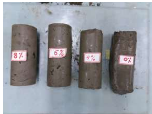
Fig. 5. Results freezing test of different type of clay samples.
