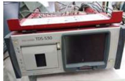
Fig. 2. Monitor to check displacement freezing soil
