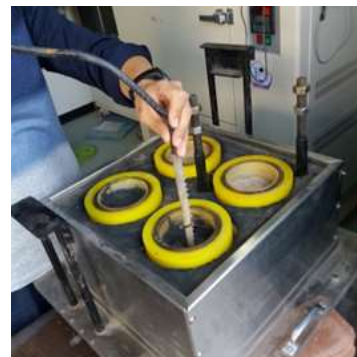
Fig.3. Prepare soil in samples for freezing test
