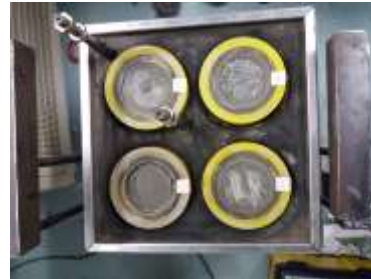
Fig. 1 Four samples in freezing box
