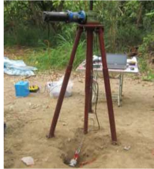
Fig. 2 Pullout apparatus for plant roots.
