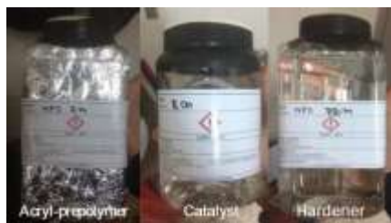
Fig. 2. The composition of the acrylate-cement grout.
