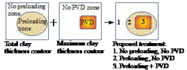
Fig. 3. Approach to determine treatment methods for ground improvement projects
