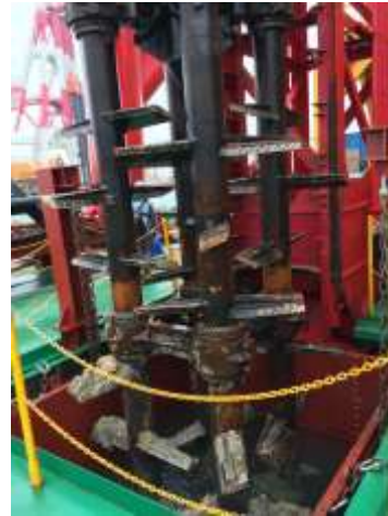
Fig. 2. Augers of a drill rig on barge
