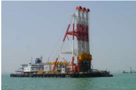
Fig. 1. Deep cement mixing barge
