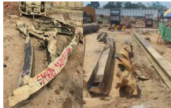
Fig. 11. Bent and twisted piles
