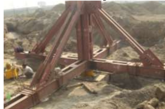
Fig. 3. Set-up for footing load test
