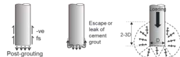
Fig. 10. Shaft Friction and End Bearing (Kentledge Test).
