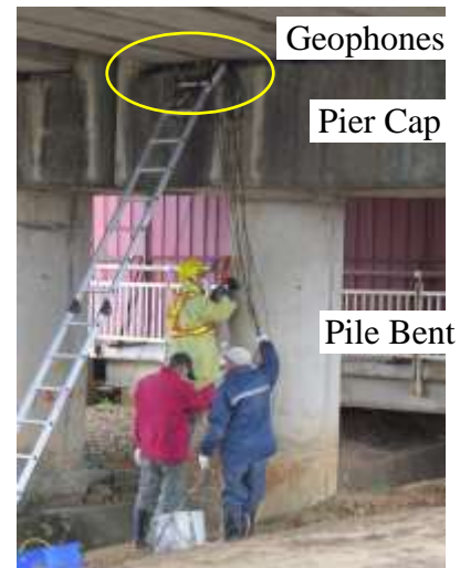
Fig. 7. Flexural impulse response conducted on a pile bent.
