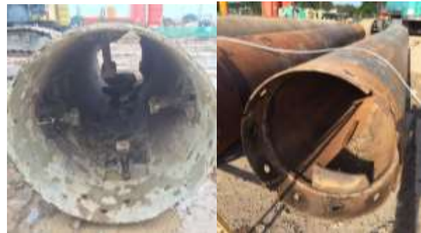
Fig. 10. Casing with clamp and blade
