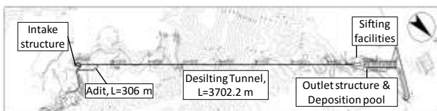
Fig 7. Plan view of the sediment desilting tunnel at Shimen Reservoir
