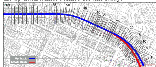
Fig. 2. Distribution of 69 sections along the up-track tunnel
