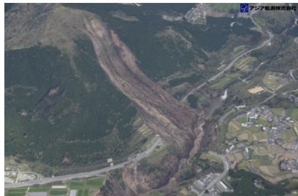
Fig. 1. Deep-seated landslide due to the 2016 Kumamoto earthquake in the Tateno district of Minamiaso village. This photograph was taken by Asia Air Survey Co., Ltd.
