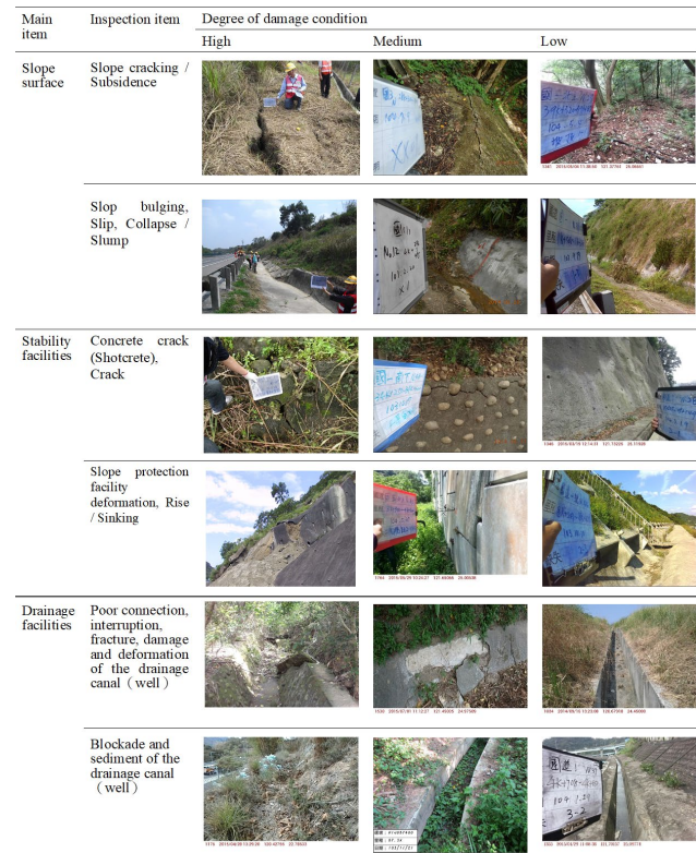
Fig. 1. Photos of degree of damage conditions for some inspection items.
