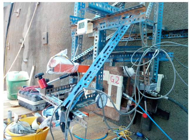
Figure 3. Typical Setting Up for Pull Out Test
