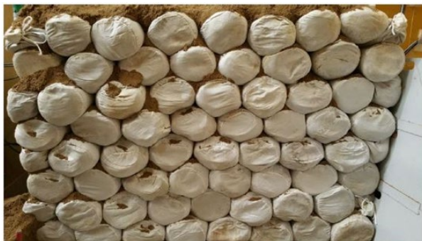
Fig. 11. Soil-bag stacks after the shaking test (750Gal).
