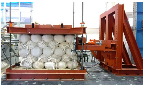
Fig. 3. Shaking test of soil-bag stacks considering the lateral pressure from the embankment.
