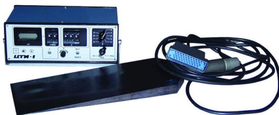
Fig.1. Wedge dilatometer WD-100:
