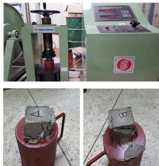
Fig. 3. Laboratory uniaxial strength test of admixture.
