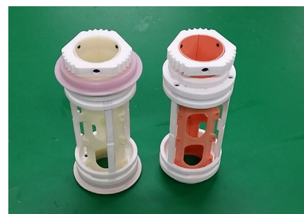
Fig. 7. Sealing packer prototype developed for this test.
