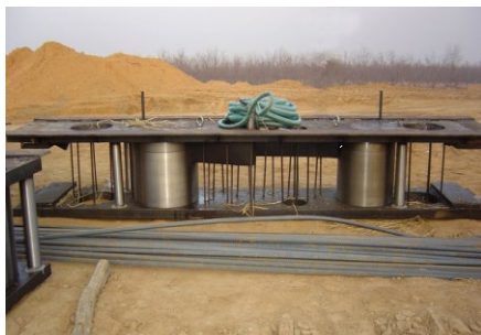
Fig. 3 One piece of rectangular loadcell
