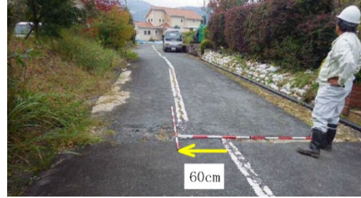
Photo. 2. Horizontal crack displacement, 60cm at point (a)
