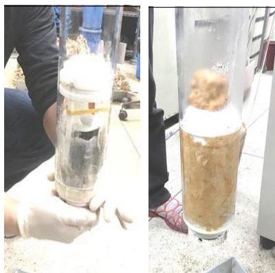
Fig. 4. Putting packer with admixture into acrylic tube and foaming scheme.
