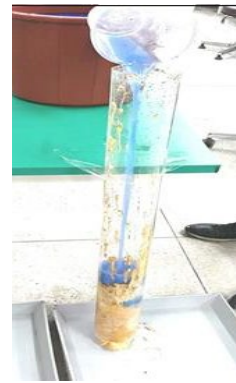
Fig. 5. Leaking tests of packer (12 hours after foaming).
