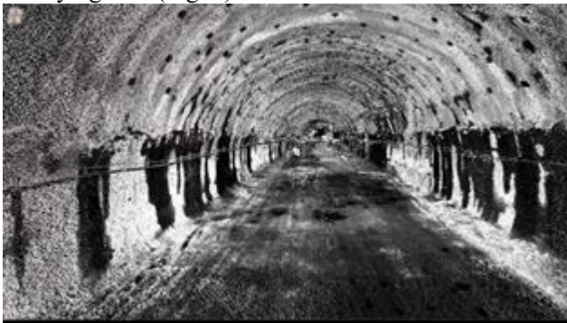
Fig. 6. 3D LiDAR scanning schematic and spatial three-dimensional information.
