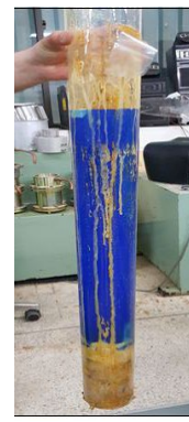
Fig. 5. Leaking tests of packer (12 hours after foaming).
