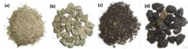
Figure 23. (a) Fine RCA; (b) Coarse RCA; (c) Fine RAP and (d) Coarse RAP used in the Geobarrier system
