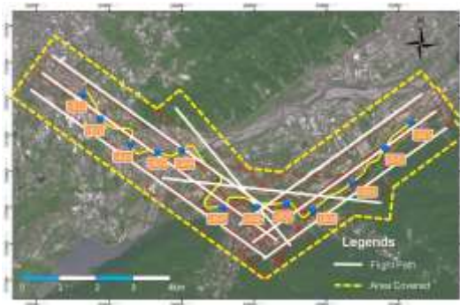
Fig. 14. Paths of UAV flights for the preliminary survey of Sanyin Line
