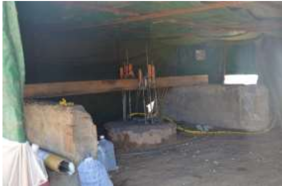
Fig. 5. Bi-Directional static load test in construction site.
