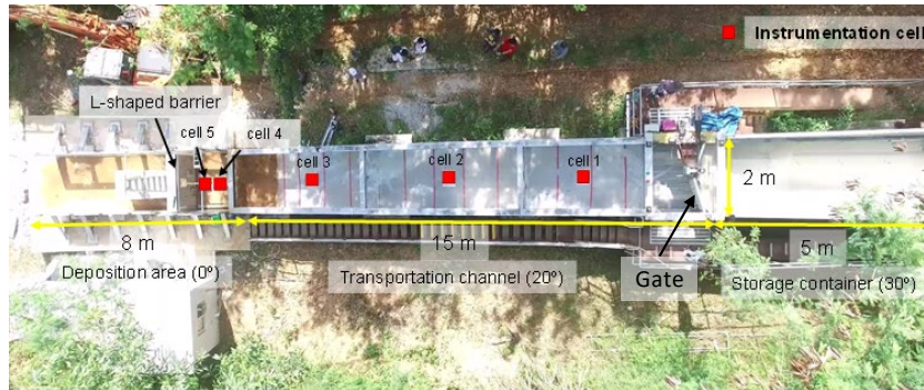
Fig. 5. Plan view of the 28 m-long flume model
