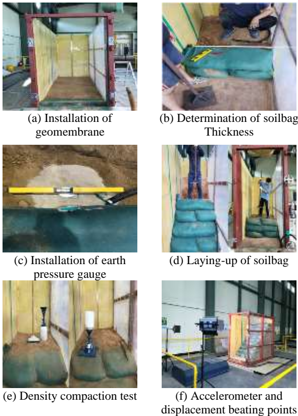
Fig. 7. Shaking table test set-up of soilbag retaining wall
