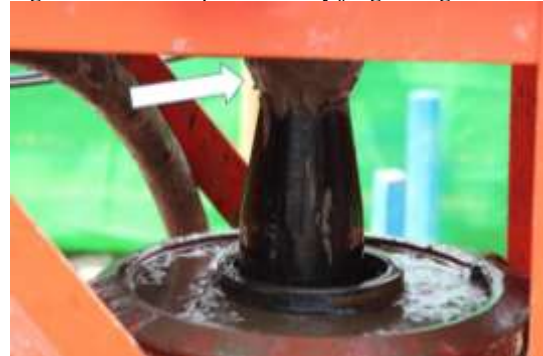
Figure 5 Jet grouting machine whose operation was stopped by plastic drains
