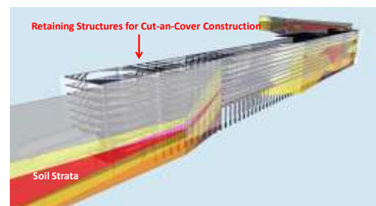
Fig. 24. BIM model of temporary works of excavation at R03 Station
