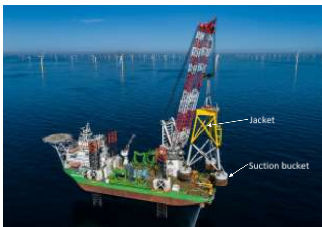
Fig. 1. Offshore wind turbine supported by suction bucket jacket (source: DEME Group).
