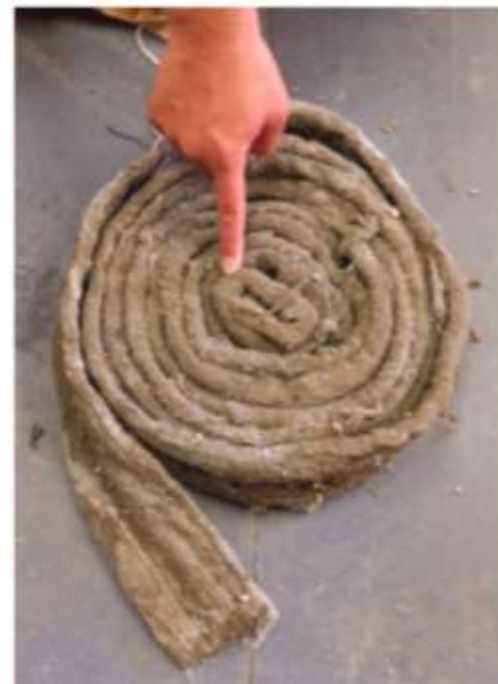
Figure 6 Plastic drain that disturbed jet grouting
