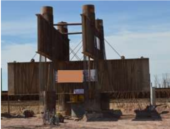
Fig. 3. Static top-down load test in construction site.
