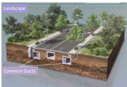
Fig. 10. BIM models for landscape and underground utilities
