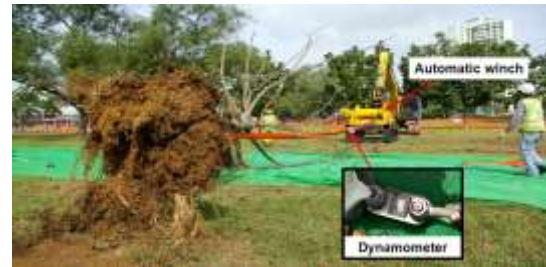
Figure 30. Tree pulling test set up in the field
