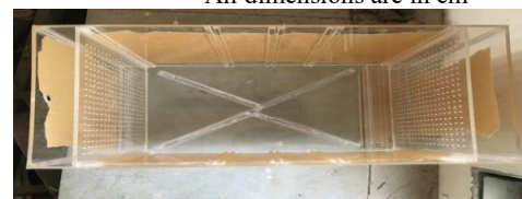
Fig. 1. Schematic sketch of model for Electro-kinetic test and actual model
