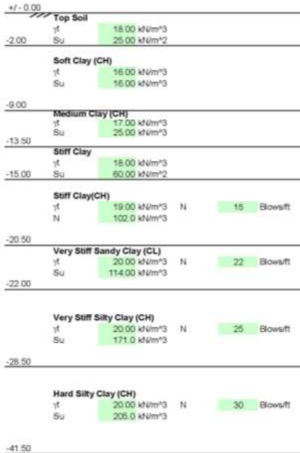
Fig. 2. Soil Profile and engineering properties
