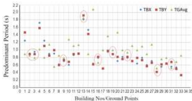
Fig. 4. Comparison of fundamental periods of the target buildings and predominant periods of nearby free-field [TBX: fundamental period of the buildings in longitudinal direction; TBY: fundamental period of the buildings in transverse direction; TGAvg: average predominant period of the free-field].
