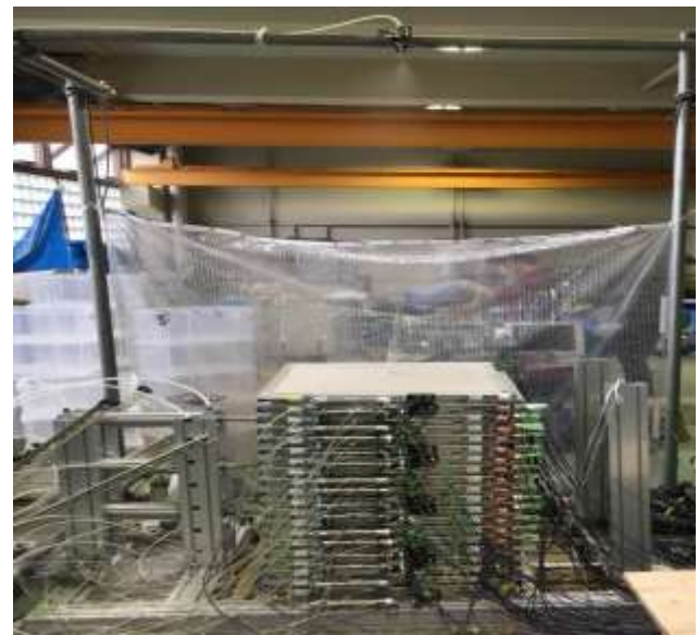
Fig. 1. Multi-layered shear model test apparatus
