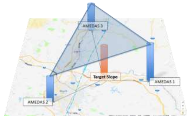
Fig.2. Estimation of rainfall data of target slope
