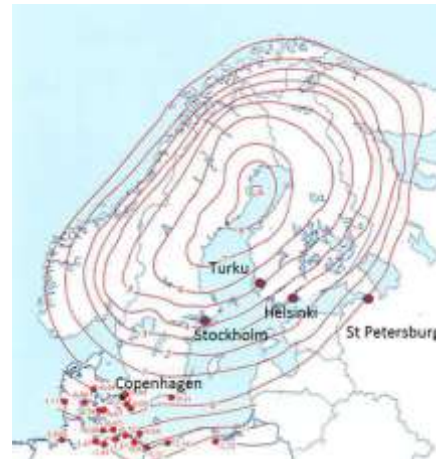
Fig.4. Isolines of modern velocities (mm/year) of the post-glacial uplift for the Fennoscandian region (Ekman, Rosentau et al.)
