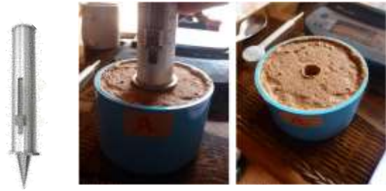
Figure 11 Strength test by Yamanaka Cone with time The results are shown in Figure 13, which indicates an amazing increase of strength of 60 times or 6 MPa of one bearing strength.
