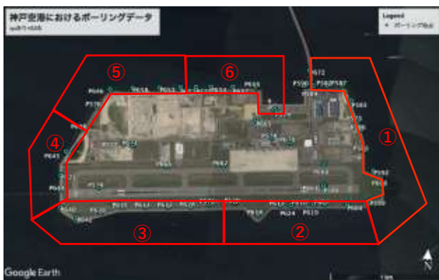
Fig. 2. Locations of soil investigations along with construction section for reclamation revetment
