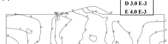
Figure 4 Influence of cohesion on incremental shear strain in dykes
