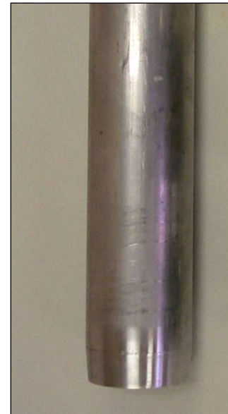
Modified thin-walled (Shelby) tube
