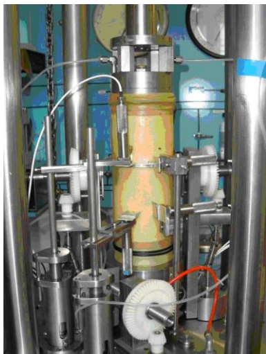
Local small strain measurement systems (after Ibraim et al. , 2011)
