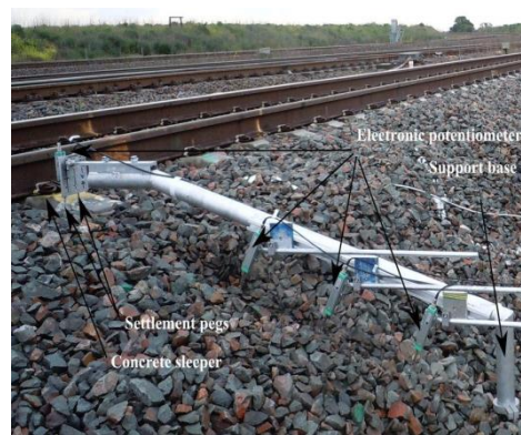
2. Track Displacement Monitoring (Indraratna et al , 2014)
