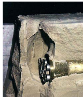
Unsupported cavity (After König et al., 2014)
