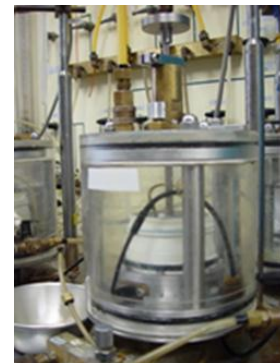
(b) View of the consolidation cell
