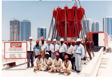
3000 t Load Test with Reaction Anchors
