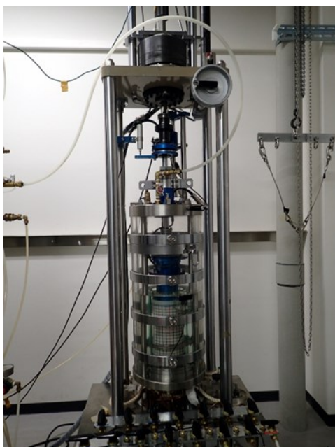
Triaxial cell of hollow cylinder torsional shear apparatus (After Toyota, Le and Takada, 2019)
