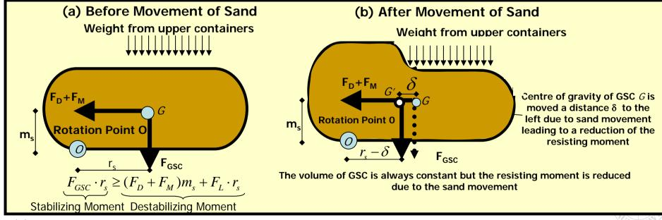
(b) Effect of the Internal Movement of Sand on the Overturning Stability of a Sand Container
