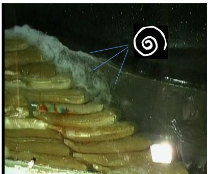
**Well-structured vortices** characterized by fluid particles moving around a common centre. These vortices appear in the areas between containers.
