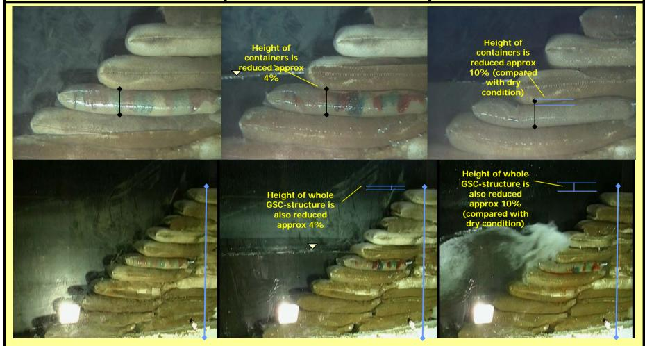
Conclusion: Initial height of the GSC-revetment is reduced approx 4% due to wet conditions and 6% due to wave action, leading to a total reduction of the height of the GSC-structure of about 10% as compared with dry conditions
