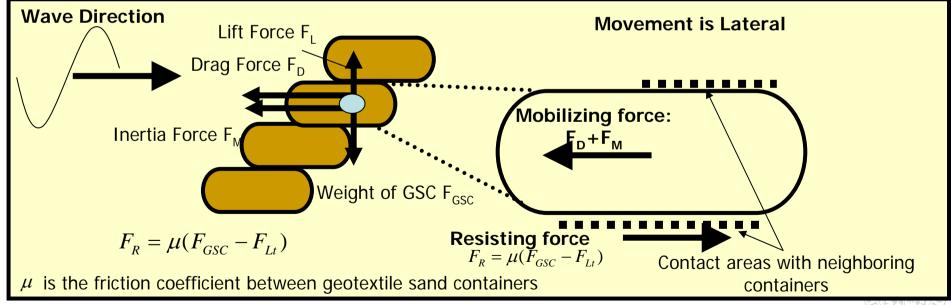
(b) Hydraulic Stability of a Sand Container against Sliding without Deformation
