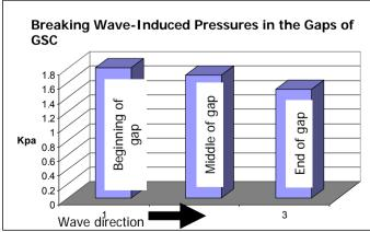
Pressures along the gap between containers are reduced (dampening due to flexibility of containers)
