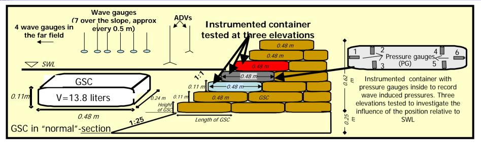
(a) GSC-Structure in the Wave-Flume (adjacent to PIV-measuring section)
