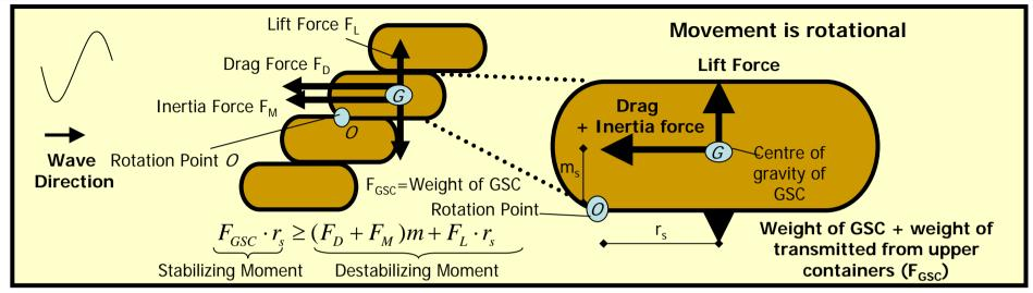
(a) Stability of a GSC against Overturning without Deformation
