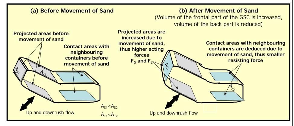
(c) Effect of the Internal Movement of Sand on the Sliding Stability of a Sand Container
