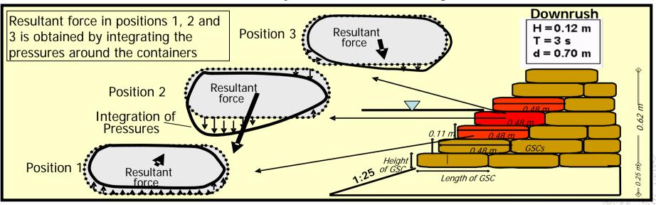
(b) Wave-Induced Loads on Instrumented Sand Container During Wave Down Rush
