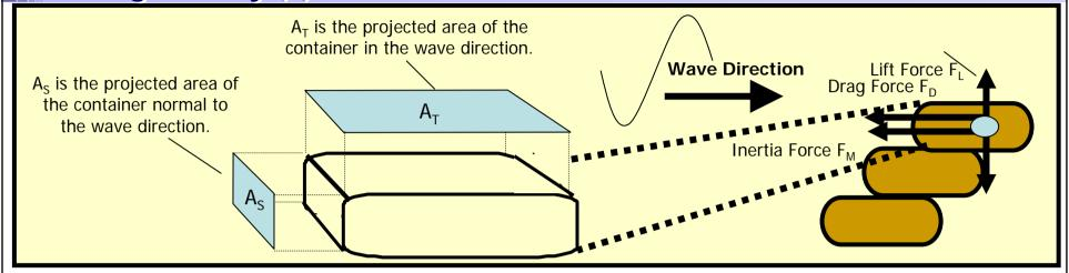
(a) Projected Areas A<sub>S</sub> and A<sub>T</sub> of a Sand Container without Deformation
