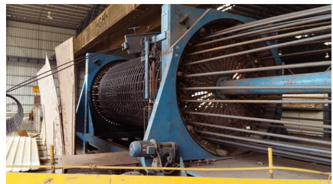
Figure 5 Template of monopile reinforcement
