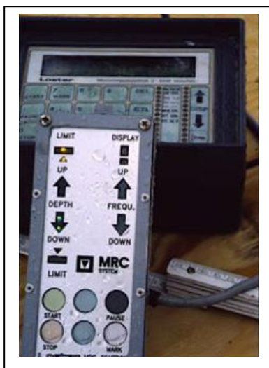
Figure 2. Interactive display that guides the machine operator during the resonance compaction process showing compaction Monitoring and Process Control of Vibratory Driving by K. R. Massarsch and C. Wersäll
