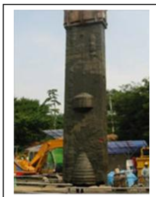
Left: Photo 1 Test nodular diaphragm wall having nodular parts and pile base enlargements Right : Figure 1 Alternative of foundation types In-situ Full Scale Load Tests and Estimation Method of Pile
