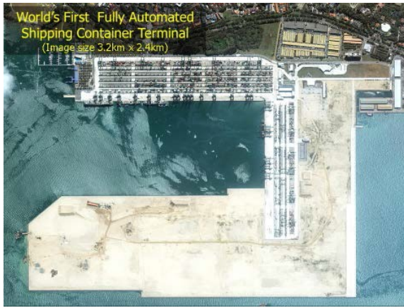
Pasir Panjang Container Terminal - ground improvement includes PVD + Surcharge vibro, deep sand compaction and dynamic techniques
