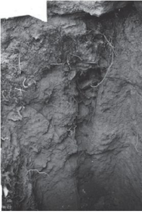
Figure 15. Infilled tension crack
