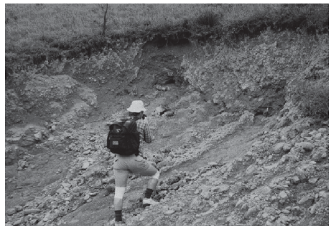
Figure 10. Failure involving surface mantle of colluvium
