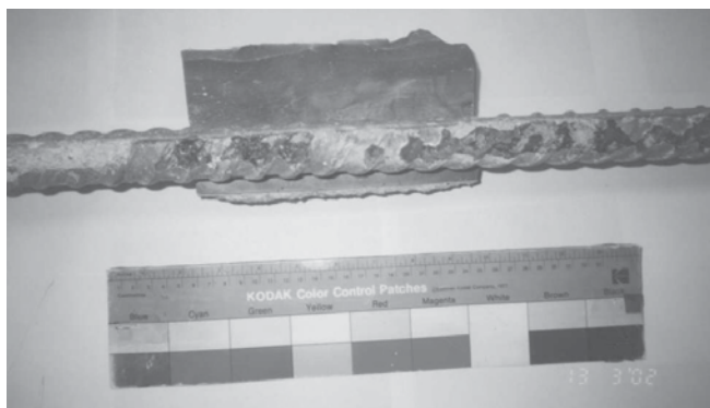
Figure 21. Localized corrosion in exhumed soil nail
