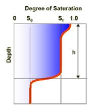
The intensity of surface infiltration is generally proportional to rainfall density but affected by the runoff characteristics of the ground. The wetting band thickness that forms as a result of rainfall is also related to the initial degree of saturation of the soil mass. Thicker wetting bands are therefore more likely to occur in wet season than after dry spells.
