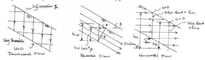
Areas of parallel downward flow are where inflow from the uphill area = outflow to the downhill area - no surface infiltration and no leakage from the base. We may make use of the concept of flowlines and equipotentials from flownet analysis to appreciate distribution of pore water pressure in the hillside.
