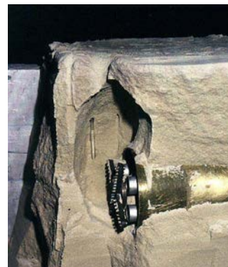
Unsupported cavity (After König et al., 2014)
