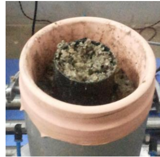
Figure 1 (a): Geocell sample prepared
