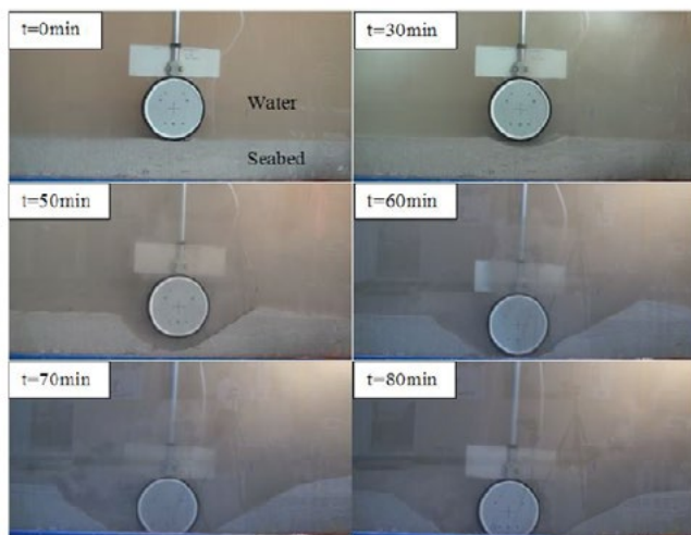
Seabed mobility and pipe movement modelled in the Large O-tube flume (After Luo et al., 2014)
